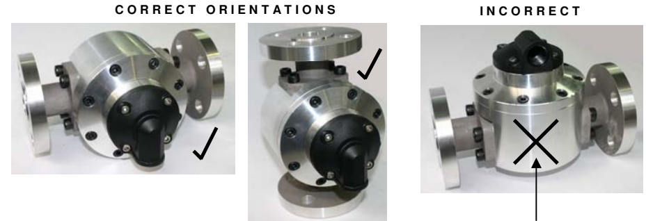
When installed incorrectly the weight of the rotors will bear down on the base of the measuring chamber.
